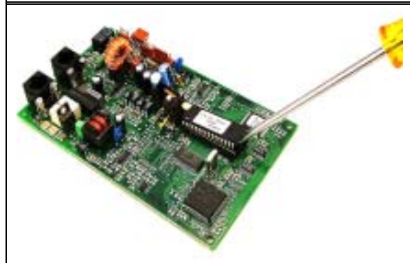
Figure 1: Removing the ROM
